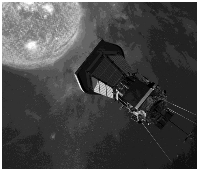
The Solar Probe Plus spacecraft with solar panels folded into the shadows of its protective shield, gathers data on its approach to the Sun. (JHU/APL)
